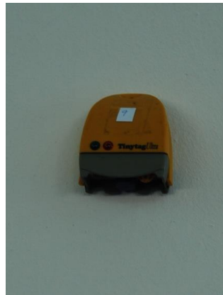
Figure 4. 16- 'Tinytag' data logger to measure the air temperature and relative humidity
