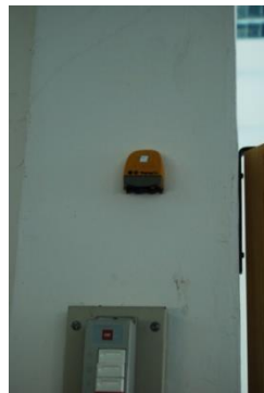
Figure 4. 17 – The data logger is placed at one metre high from the floor level
