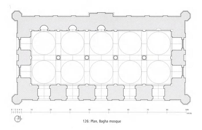
compound surrounded by a low wall. It is accessed through two arched gateways from the north and south. A big tank was dug on the eastern side. This mosque was seriously damaged in the earthquake of 1897 when all the domes and the eastern wall collapsed (S. Ahmed 1960:213). The praiseworthy restoration was undertaken in 1978 by the Directorate of Archaeology Bangladesh.
