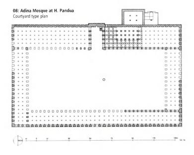
the iwans. The Adina mosque, built in 776-86A.H./1374-84A.D. at Hazrat Pandua, (A. Ahmed 1997:142) is the single example of the courtyard-type mosque in Greater Bengal (Plate 08). The large courtyard or sahn (127.7 x 57.2 m) is surrounded on three sides with riwags and with the kibla riwag on the fourth side. This type of large monumental mosque with inner courtyard was never repeated anywhere else in Bengal.
