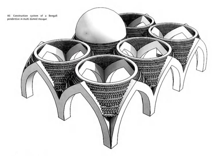
only at certain specific points. As a result of this practice outer surface or the extrados of the dome shows a series of steps. Accordingly the surface finish does not have a regular or smooth curve but follows the structural configuration of the dome. The Chakmatti mosque (Plate 47) and the Latton mosque at Gaur have stepped extrados.
