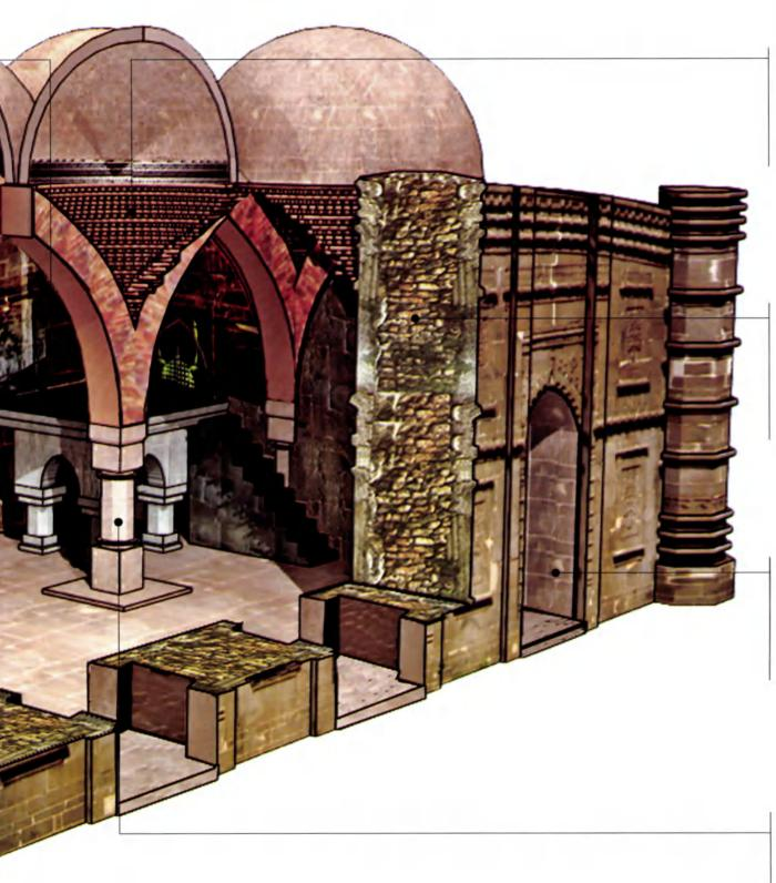
Bengali pendentive Corbelling and diagonally placed brick layers are placed alternately to transfer the square supporting area into circular base for the dome.
