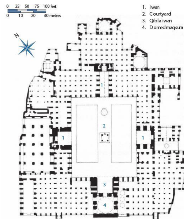
Figure 5: Plan of the Great Mosque of Isfahan, Iran, showing four iwans opening onto the sahn (court) ( https://classconnection.s3.amazonaws.com/650/flashcards/4706650/jpg/a9rafe1-145143EFC7E1544A799.jpg )
