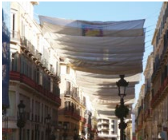
Fig. 2 Textiles stretching from one façade to the opposite to create shadow in Larios street, Málaga, Spain (photo: F. Vegas, C. Mileto).
