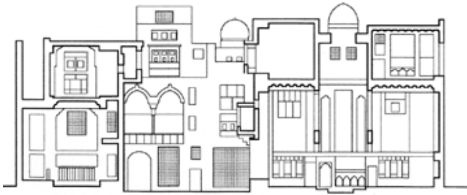
Fig.7 Section of a courtyard house in Cairo, Egypt (drawing: A. Picone).
