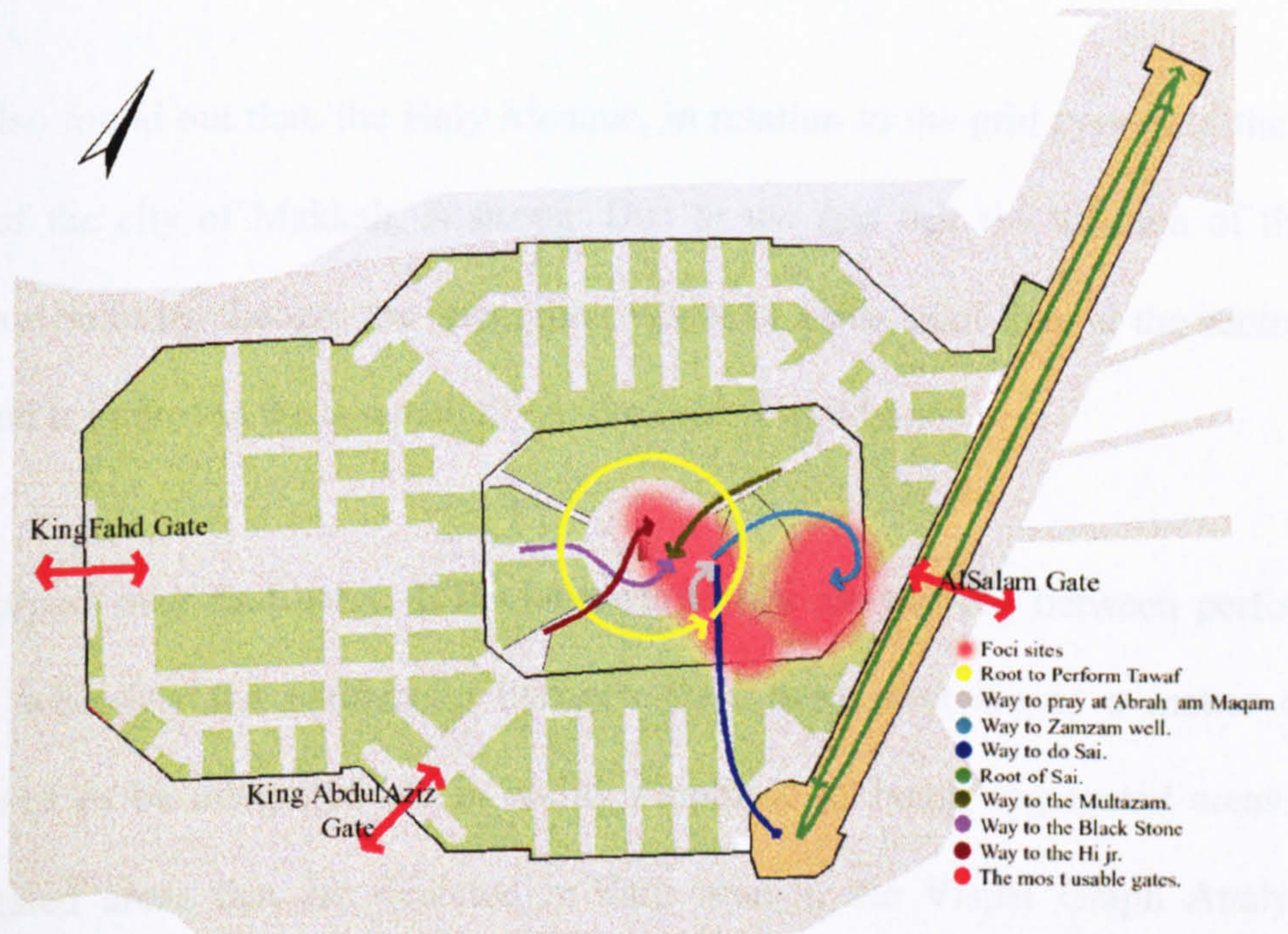
Figure 7- 25: A graph showing the most efficient routes for fixed activities inside the Holy Mosque building with the location of the fixed elements and the most convenient gates allocated. Praying could be performed at any place inside the mosque however, the green sites is the assigned area for praying.
