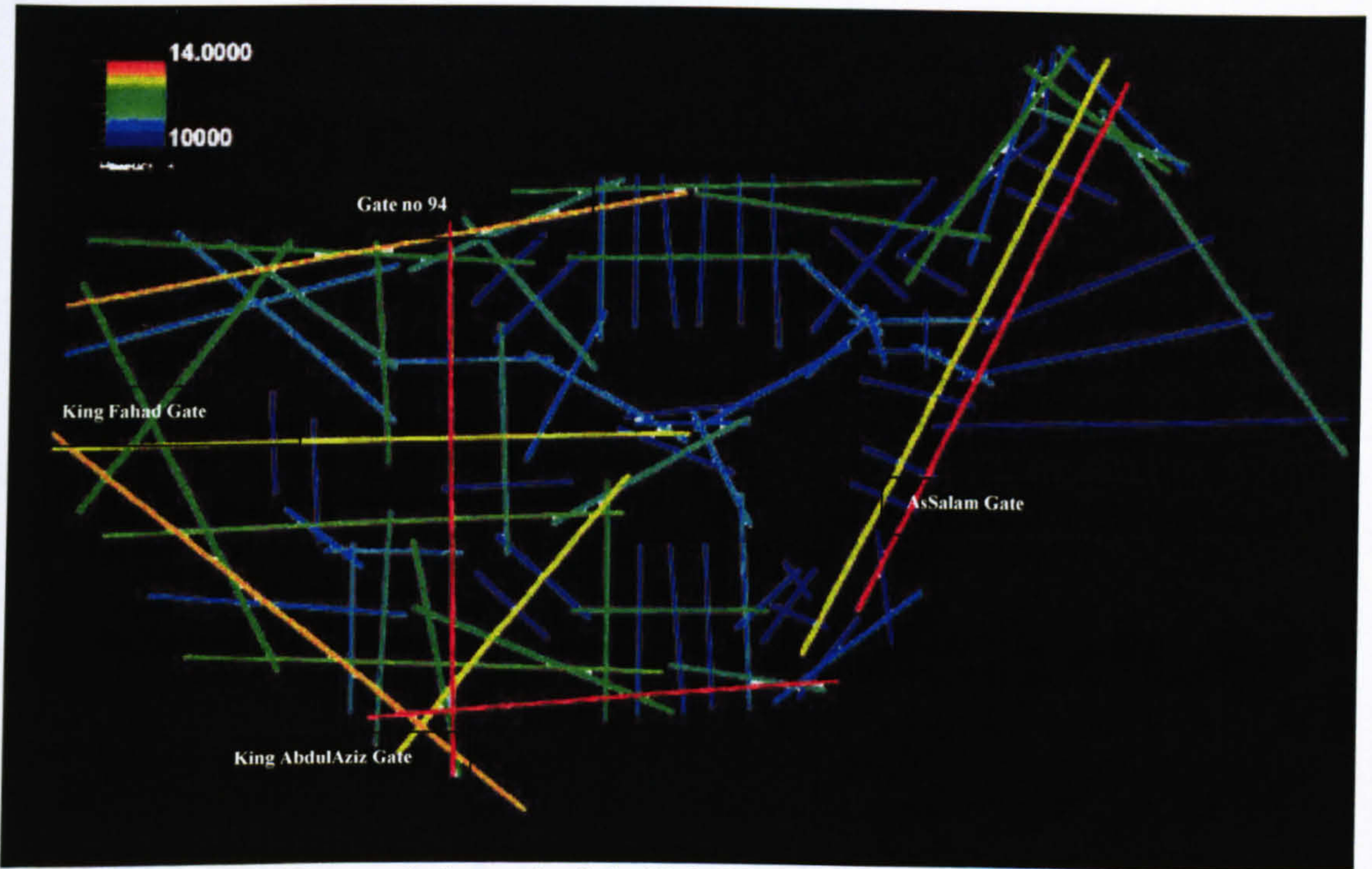
Figure 7- 12: Axial line analysis graph of the Holy Mosque, showing the axial lines connectivity.
