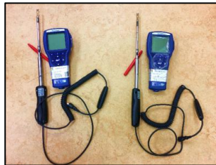
Fig. 3. The two sets of multiparameter ventilation meters namely TSI Velocicalc 9565 series.
